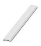
Zack Marker strip, flat, Strip, white, unlabeled, can be labeled with: PLOTMARK, CMS-P1-PLOTTER, mounting type: snap into flat marker groove, for terminal block width: 12 mm, lettering field size: 5.15 x 12.15 mm
