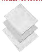
Steel panels are 14 gauge, finished with white polyester powder paint or with a conductive, corrosion-resistant coating. Stainless steel panels are 14 gauge Type 304 and have a commercial #3 finish which is protected on one side with a plastic film. Aluminum panels are 5052-H32 aluminum alloy 0.080-in. (2-mm) thick and protected on one side with a plastic film. Panel mounting hardware is furnished with all enclosures which accept these panels.
