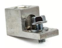
350 kcmil-6 AWG wire range, and FLEX wire class G-K including mm2 class 5, 1 barrel, aluminum or copper wire, CU9AL, 90C temperature rating, one mounting hole of .343 inch dia 5/16" bolt, UL Listed, CSA Certified.
