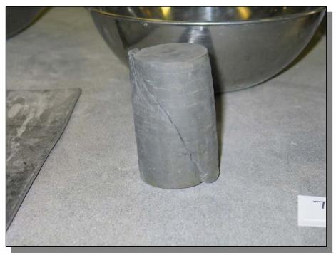
b. Sample TB-2C No. 16 (AP-611-MW) after testing. Note failure plane.
