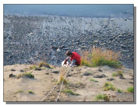
b. Measuring water flow from the bluff at Soil Profile SP-E. The procedure involved catching the flow and then measuring in a bucket. October, 2006. 03 of Appendix A. Soil profile locations are also shown on the annotated photo mosaic presented as Drawings A-08 through A-10.
