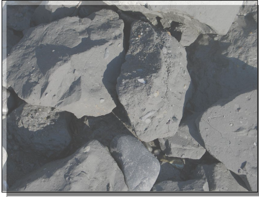
a. Large chunks (boulders) of clay found at bottom of bluff. From a distance, these chunks can be mistaken for cobbles and boulders. October, 2006.
