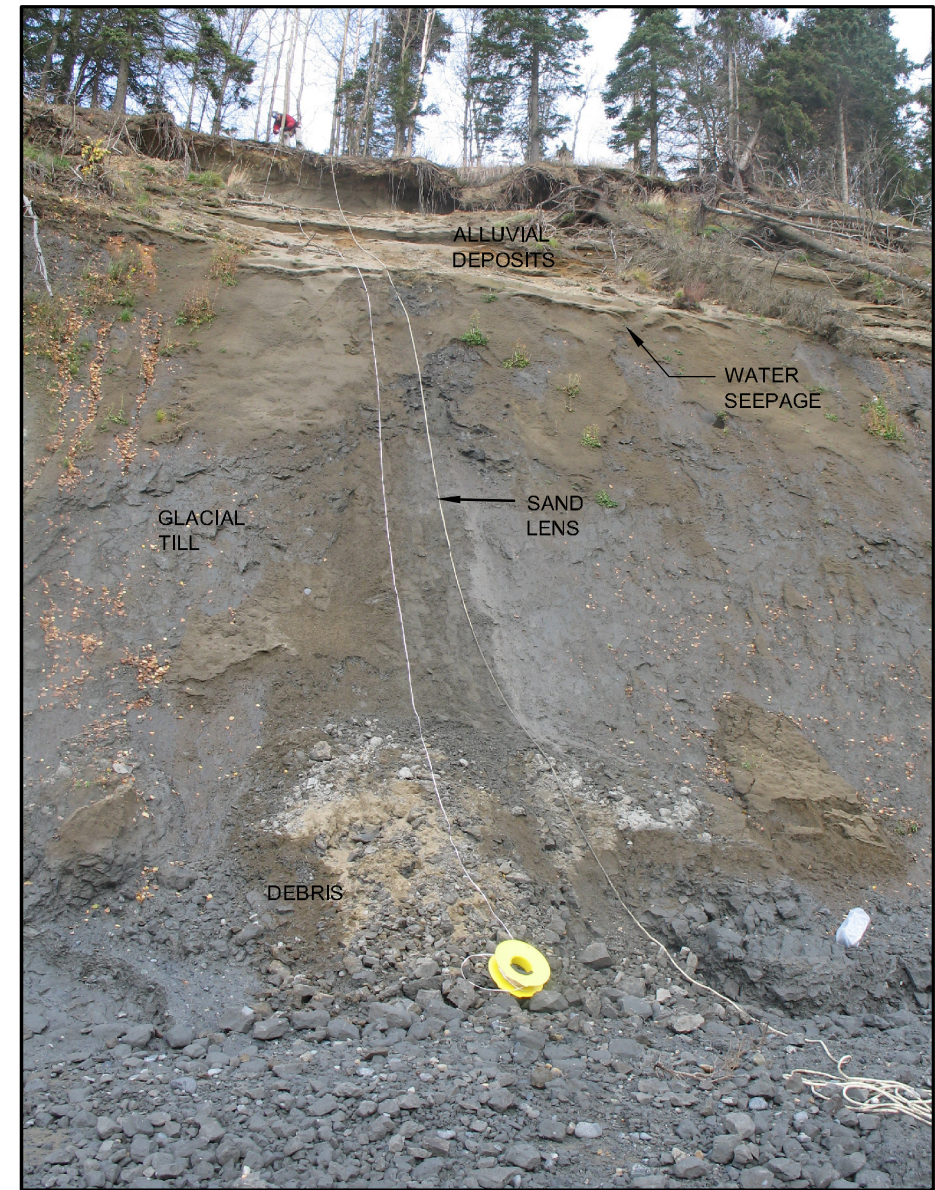
LOOKING NORTH AT SP-G. MOST OF THE EXPOSURE IS COVERED BY A THIN LAYER OF SAND. NOTE CHUNKS OF DARK GRAY CLAY AT BASE OF SLOPE. 10 OCT. 2006
