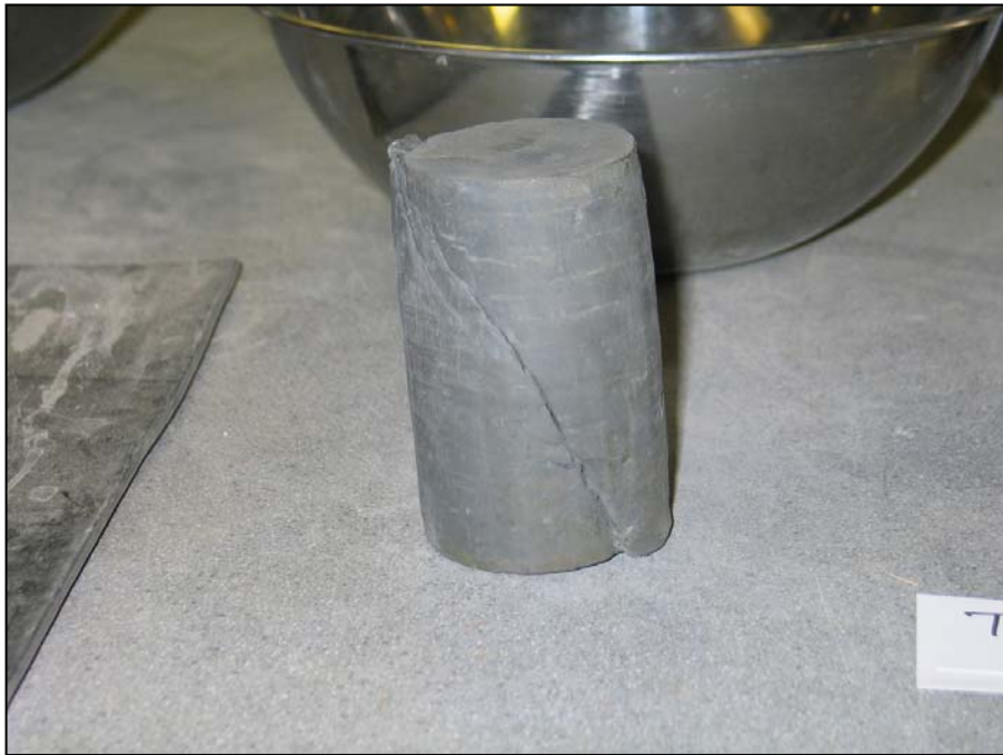
b. Sample TB-2C No. 16 (AP-611-MW) after testing. Note failure plane.
