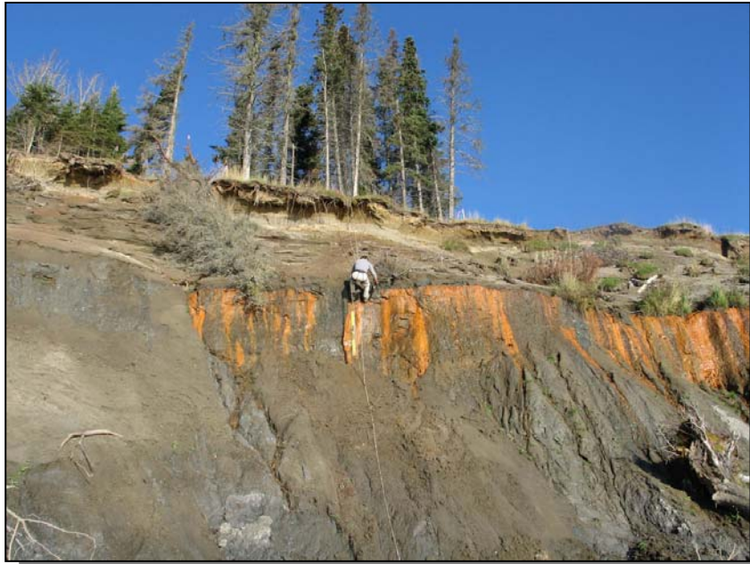
a. Rappelling down the bluff face at Soil Profile SP-D. The four-foot yellow electronic level was used to measure slope angle. Slope distances were measured using the white tape. October, 2006.
