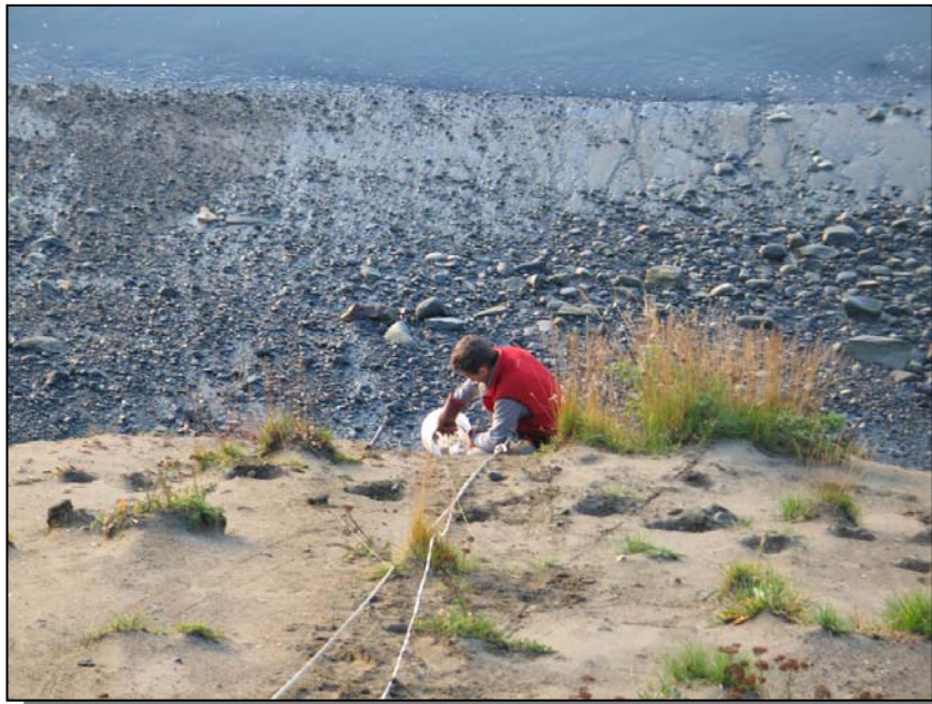
b. Measuring water flow from the bluff at Soil Profile SP-E. The procedure involved catching the flow and then measuring in a bucket. October, 2006.
