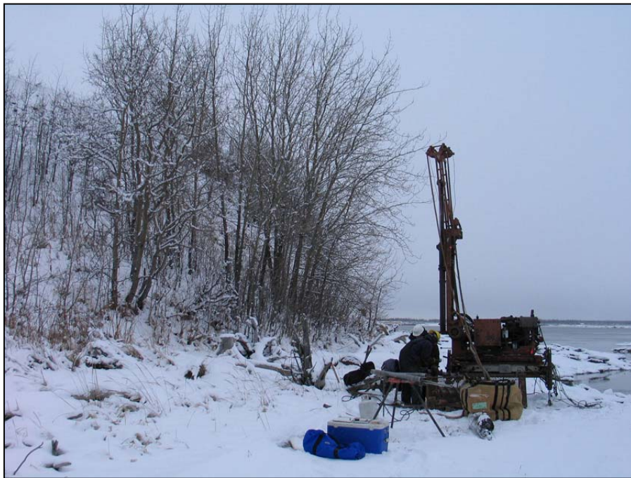
b. Drilling at Test Boring AP-622 with helicopter portable drill rig. December, 2006.
