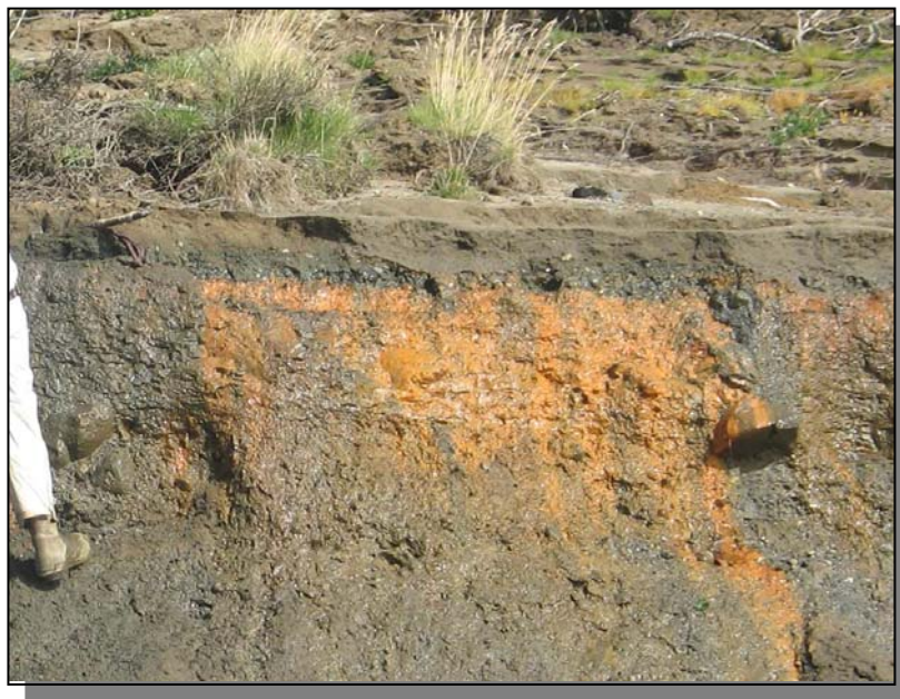
b. Thin layer of lag gravel near Soil Profile SP-H. Layer ranged from two to six inches thick and can be seen between the rust stained glacial till below and brown sand above. Water was observed flowing out of the gravel at this location. October, 2006.
