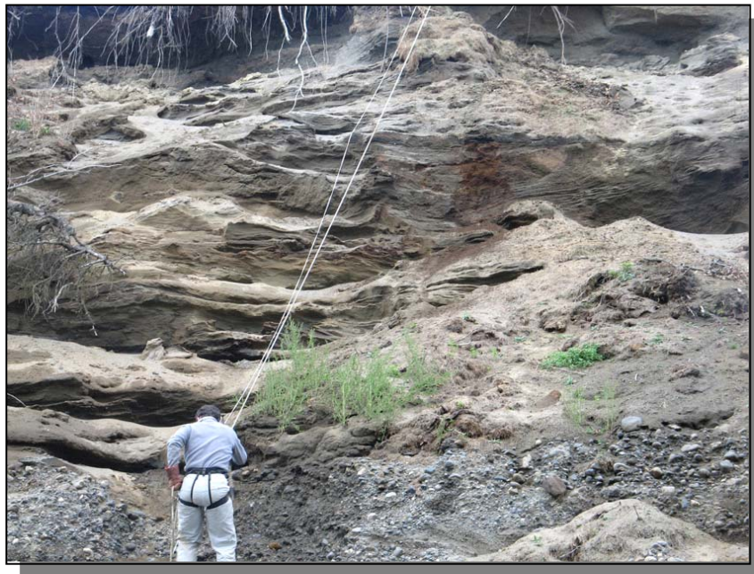
b. Cemented layers of sand at Soil Profile SP-C. Cementation appears to allow the sand to stand almost vertical. October, 2006.
