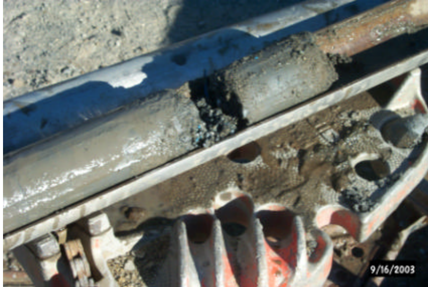
Photograph 3 – Small 2-inch sand seam within lean sandy clay
