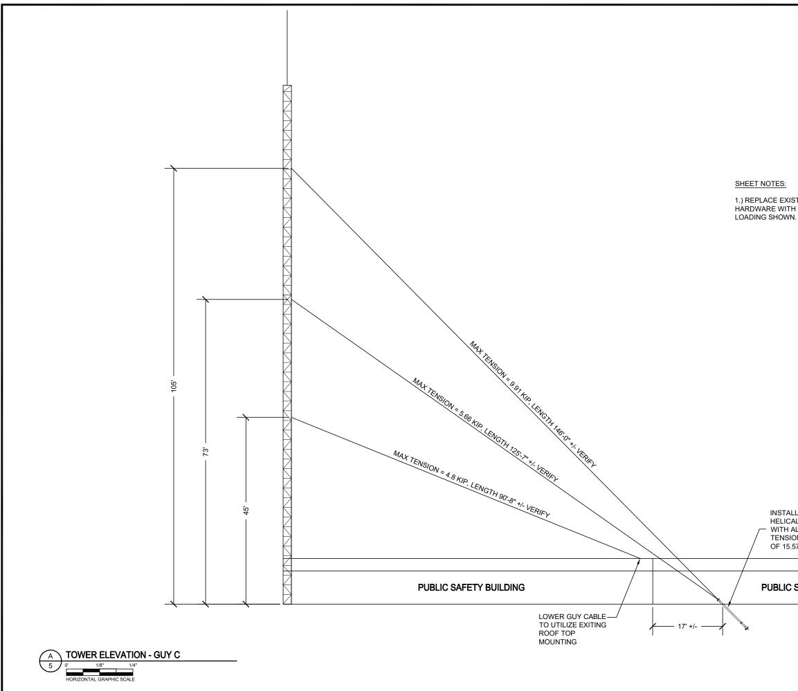
1.) REPLACE EXISTING GUY WIRES AND CONNECTION HARDWARE WITH MATERIALS SIZED FOR THE TENSION
