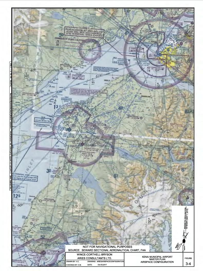
There are two global positioning system (GPS) approaches. They are RNAV (GPS) to Runway 1L and RNAV (GPS) approach to Runway 19R. (RNAV approaches rely on aircraft area navigation equipment.)
